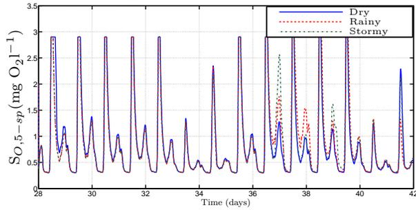
Fig. 6: Comparison of obtained optimal set points using Method5.
