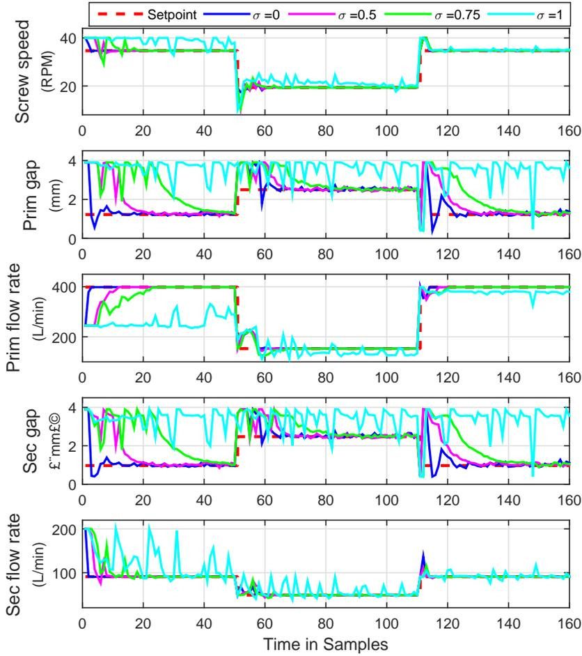
Figure 7: The manipulated variables of the MP process for Example I
