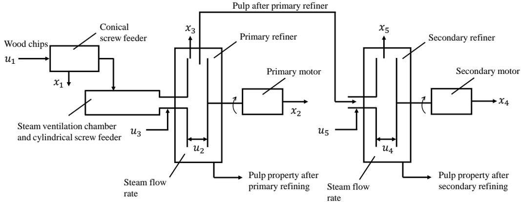
Figure 2: Schematic of two-stage HC refining
