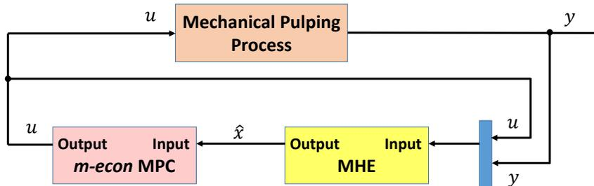
Figure 3: Graphical depiction of the integrated *m-econ* MPC and MHE for MP process
