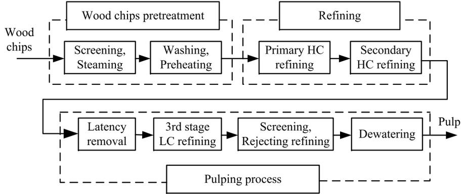
Figure 1: Operational units in a typical two-stage MP process
