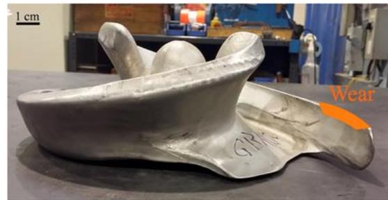
Fig. 1. A two-blade centrifugal pump impeller used for moving a slurry of water and paper pulp. Erosion often manifests in the region denoted in orange.
