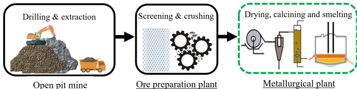
Figure 1. Simplified illustration of the relevant mining and metallurgical processes
