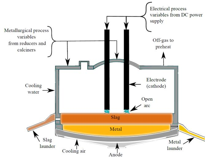
Figure 2. Schematic of a direct current electric arc furnace.
