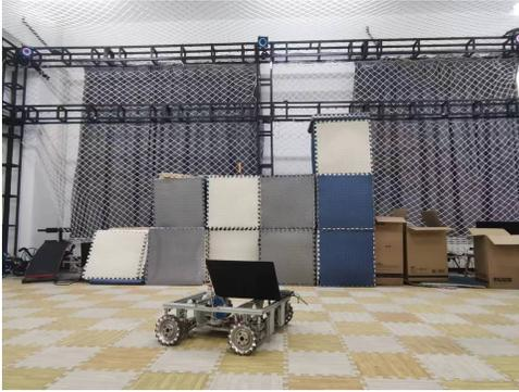
Fig. 4: Experiment overview. The field is  $6 \times 8$  m, with 8 cameras on top of the field capturing the pose and position of the robot. A target for the capturing system is fixed on the side of the robot.
